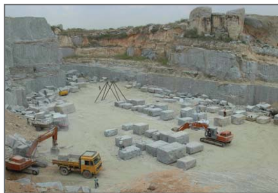
Fig. 3.7: Quarrying of limestone
